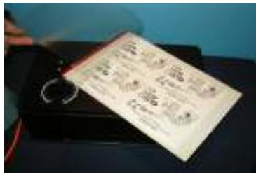
There are two types of thermal copiers - belt & roller types - the steps described below will vary slightly according to the type and brand of thermal copier being used. These instructions are for roller type VistaFax models [1UF model pictured].
